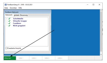
The loudspeakers in the Pan Beam series are to be set up through the Pan Beam Setup software. The Dante Controller software from Audinate must be installed to access a Dante network via the software. After successful installation, the Dante interface (Ethernet) appears in the footer of the Pan Beam Setup software.
