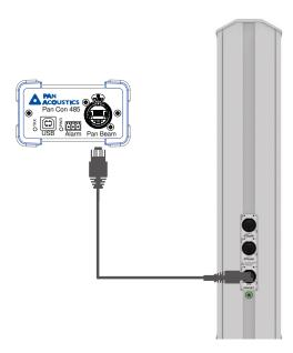
Each Pan Beam loudspeaker has an alarm contact. The loudspeaker can indicate a detected error via this alarm contact. For this purpose, a switch relay is installed in the loudspeaker, which is closed in normal operating status. If the loudspeaker is not in operation, there is no power supply. If an internal error is reported via the DSP, the relay is opened.
