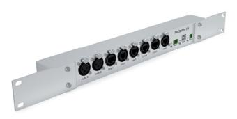
The **Pan Splitter 2/6** is a Pan Net interface with hub function that has six Pan Net outputs. The two audio inputs of the interface are available to all six Pan Net outputs. Several line arrays from the Pan Beam series can be operated per Pan Net output. In addition, the Pan Splitter 2/6 has an alarm contact and a connector for media controllers (switching of presets).
