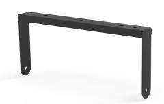
The **Swivel bracket, P 8-CX** enables the use of CX speakers from the Pan Speaker series on trusses, leaflet hoists or load bars. For mounting, e.g. a half-coupler, the bracket has a central hole [ø 11mm]. Alternatively, the bracket can be attached directly to ceilings or walls using a screw and dowel connection.
