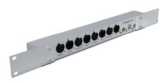
The Pan Splitter 4/4 is a Pan Net interface with hub function that has four Pan Net outputs. Each of these four Pan Net outputs has its own analogue audio input. Several line arrays from the Pan Beam series can be operated per Pan Net output. In addition, the Pan Splitter 4/4 has an alarm contact and a connector for media controllers (switching of presets).
