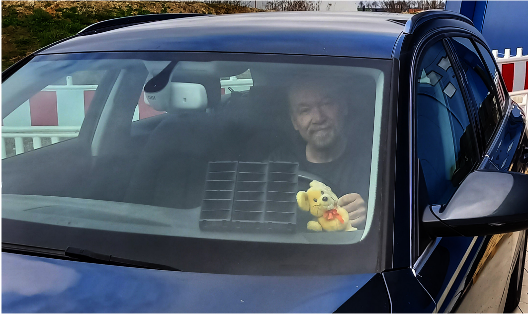
The radio transponder on the dashboard sends signals to the traffic light electronics.
